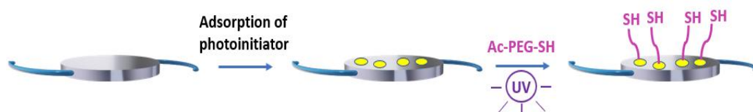
Figure 6.10: Diagram depicting the synthesis of the polymer brushes composed of Ac-PEG-SH.
