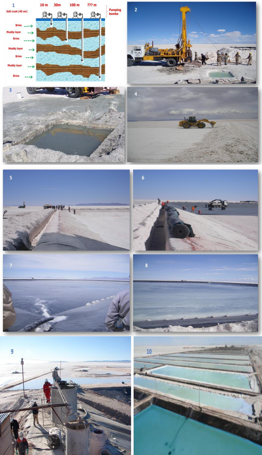
Figure 1.2. Phases for the extraction of evaporite resources in the Uyuni salt flat (Source: (GNRE (2012c), 2014))). 1. Composition of the brine, 2. Drilling of the salt crust, 3. Minerals diluted in the brine, 4. Stockpile of scarified material, 5. Building of a trench anchoring system and evaporation pools, 6. Waterproofing of pools, 7. Pumping of liquid brine, 8. Evaporation pools to let liquid evaporate naturally, 9. Whitewashing technique with quicklime, 10. Evaporation pools (In total, 16 pools in the Pilot phase in a surface of 30 hectares)
